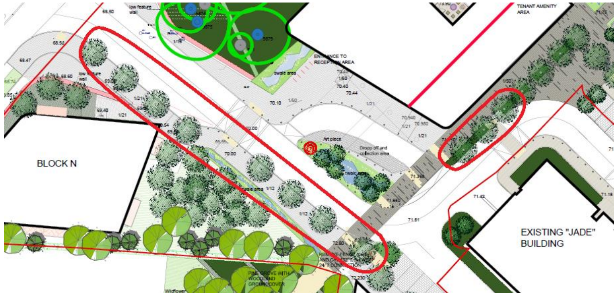
Figure 48: Trees located too close to carriageway edge
