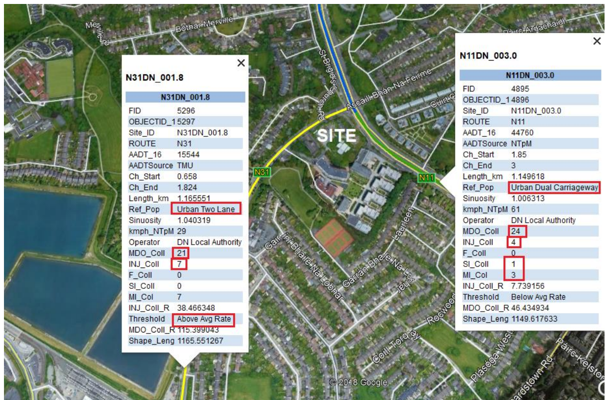
Figure 40: TII GE-STY-01022 Collision Rates 2015 to 2017 adjacent to Site
